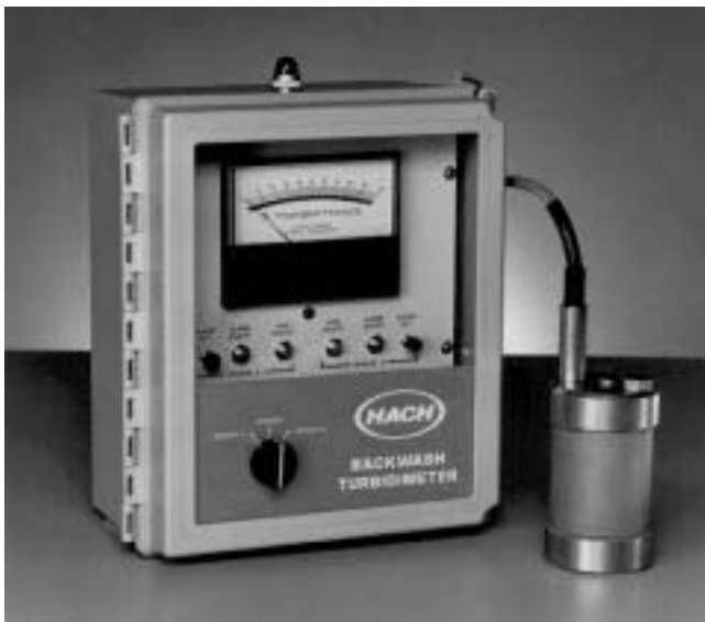
Figure 23. Hach Backwash Turbidimeter
